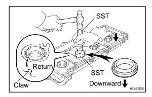
(c) Using SST and a hammer, tap in a new gasket until its surface is flush with the upper edge of the cylinder head cover.
