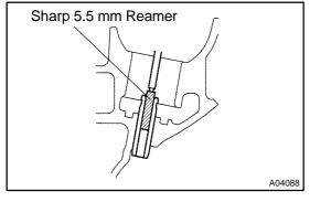
(g) Using a sharp 5.5 mm reamer, ream the guide bushing to obtain the standard specified clearance (See page EM–46) between the guide bushing and valve stem.
