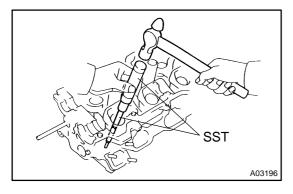
(b) Using SST and a hammer, tap out the guide bushing. SST 09201–01055, 09950–70010 (09951–07100)
