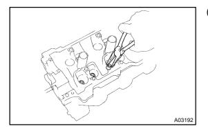
(c) Using needle-nose pliers, remove the oil seal.
