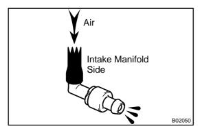
(2) Blow air into the intake manifold side, and check that air passes through with difficulty.
