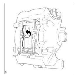
(b) Push the pin hold clip toward the brake rotor to disengage it from the brake pad, and then remove it from the 2 pad guide pins.
