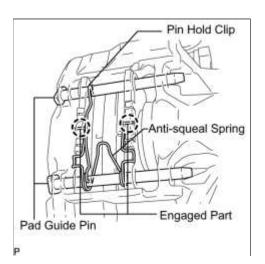
(a) Remove the pin hold clip and disengage the engaged parts of anti-squeal spring.
