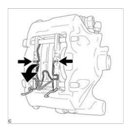
(a) Disengage the both ends of the anti-squeal spring from the 2 brake pad holes, and turn the anti-squeal spring as shown in the illustration.
