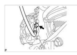
(a) Remove the union bolt and gasket from the rear disc brake cylinder, and then disconnect the flexible hose.
