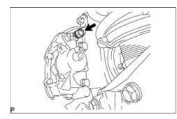
(a) Remove the cylinder slide pin and then tilt the disc brake cylinder toward the rear of the vehicle.
