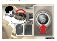
The steering lock is engaged when the driver's door is opened with the "ENGINE START STOP" switch OFF.
