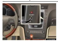
The immobilizer system prevents the engine from being started in the event that an attempt is made to start the vehicle using an unregistered key. The security indicator light flashes to indicate that the system is set.
