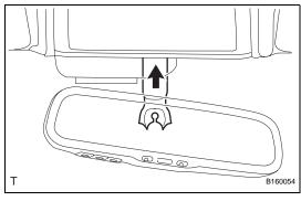
(b) Push in the cover in the direction indicated by the arrow in the illustration. Then install the cover.
