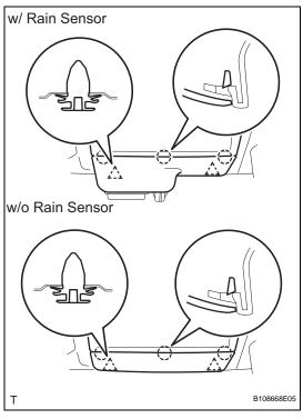
(b) Using a screwdriver, detach the 3 claws and 2 clips, and remove the top garnish.
