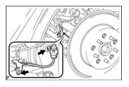
(a) Remove the 2 bolts, and separate the speed sensor from the axle carrier.
