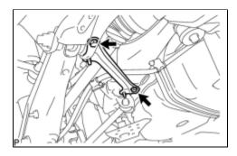
(a) Remove the 2 bolts and suspension member brace.
