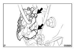
(a) Remove the 2 bolts, and disconnect the rear disc brake caliper assembly.
