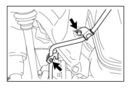
(a) Remove the 2 bolts, and separate the parking brake cable No.3.
