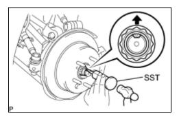
(a) Using SST and a hammer, release the staked part of the axle shaft nut.
