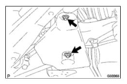
(a) Remove the 2 nuts and differential support protector No.2 from the suspension member brace.
