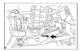
(a) Remove the bolt and nut, and separate the load sensing valve sensor bracket and stabilizer link assembly.
