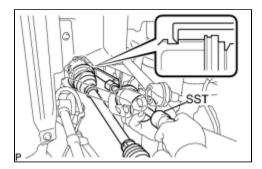
(a) Using SST, remove the rear drive shaft assembly.
