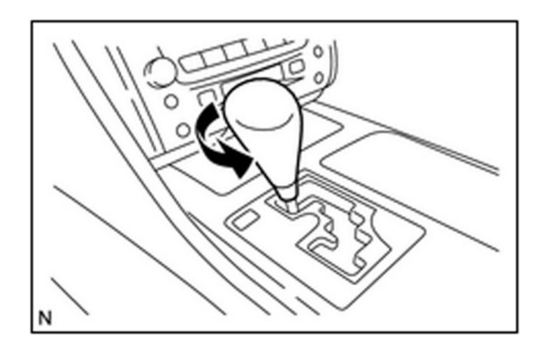
(a) Twist the shift lever knob in the direction indicated by the arrow and remove it.
