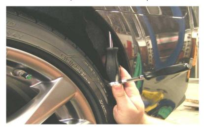
4. Underneath vehicle, remove 4x plastic fasteners and 2x 10mm screws securing edge of fascia.
