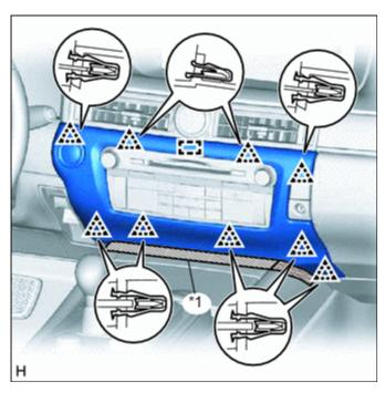
(a) Put protective tape around the center instrument cluster finish panel.
