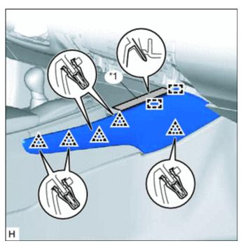
(a) Put protective tape around the instrument panel finish panel end RH.
