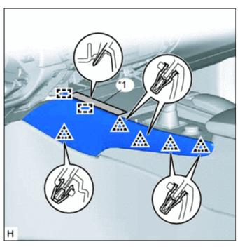
(a) Put protective tape around the instrument panel finish panel end LH.
