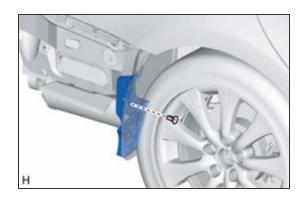
**b.** Remove the 2 screws and rear bumper No. 1 side support.
