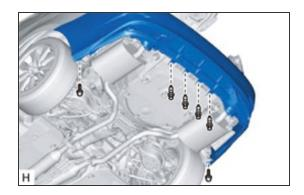
**b.** Remove the screw, and then remove the rear bumper seal bracket.
