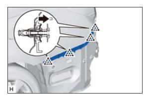
**b.** Detach the 6 claws and remove the rear bumper No. 2 side support.
