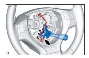
**c.** Remove the 2 screws and cruise control main switch.
