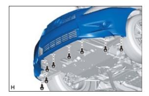
**b.** Using a screwdriver, turn the 2 pin hold clips 90° and remove the pin hold clips and screw.
