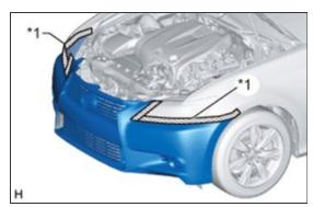
i. Disconnect the 2 headlight washer hoses and then drain the washer fluid.
