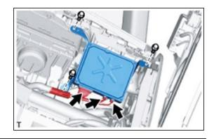
a. Put protective tape around the No. 2 instrument panel garnish sub-assembly.
