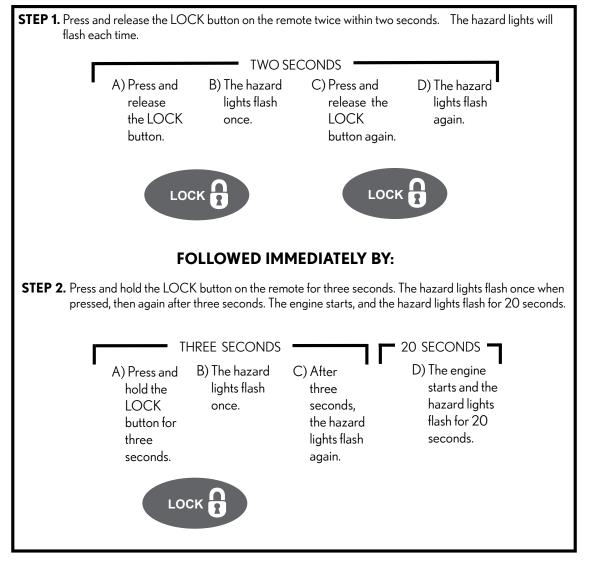
**NOTE:** Vehicles started with the Remote Engine Starter can idle for a total of 20 minutes, however automatic engine shutdown occurs after 10 minutes of run-time. You can always restart the Vehicle after this initial shutdown. Once the total run-time exceeds 20 minutes the vehicle must be manually started inorder to reset the Remot Engine Starter.
