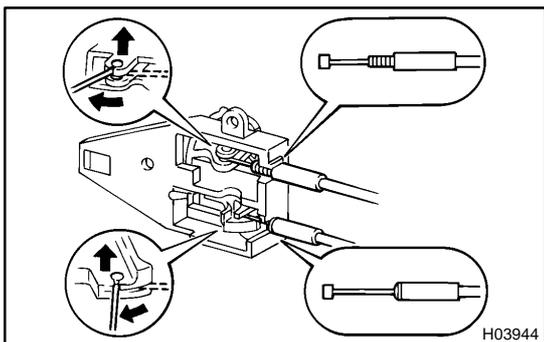
(c) Remove the 2 cables from the door inside handle.
