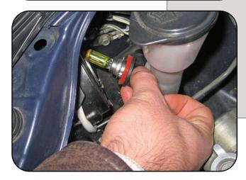
Once the bulb connector is unplugged, twist OEM bulb counter clockwise to unlock the bulb from headlight housing. Once the bulb is unlocked remove gently from housing.
