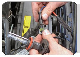
Remove the HID bulb from the protective plastic casing and screw cap. Do not touch the bulb with your bare hands. If you do, be sure to clean the bulb with rubbing alcohol prior to installation. Then Connect corresponding AMP connectors from the ballast to bulb.
