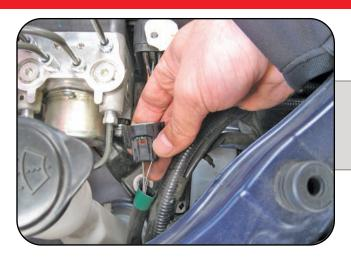
Once bulb is removed, locate your OEM bulb connector.
