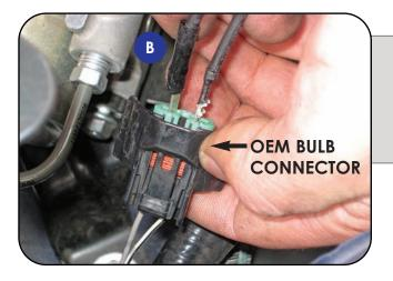
If you have the connector (B) push adapter pins into OEM bulb connector as shown on the photo.
