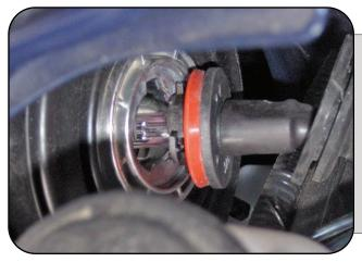
Mount ballast with the double sided tape provided to a clean flat surface in the engine bay. Twist the HID bulb clockwise to secure it in headlight housing.
