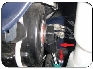
Open hood. Looking down from above into the engine bay, locate the low beam bulb. Remove retaining clip on low beam by simultaneously pushing and pulling the connector downward from the bulb.
