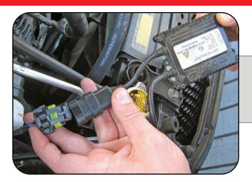
With your bulb connector now connected to the adapter, plug the 9006 end into the ballast.
