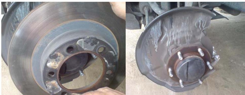
Here ensure to check the disc thickness by just running soft fingers over the face of the rotor. Here if you feel any fine lines, then you have to skim the rotors. Here I had to do it. The Toyota method is Inspection ensuring standard thickness 28.00mm and Minimum 26.00mm. so you need to skim at least 0.05mm outer edge from each side of the rotor. And that is what I did. Note: Before you skim the rotors ensure to mark the disc of each wheel as a matter of precaution..
