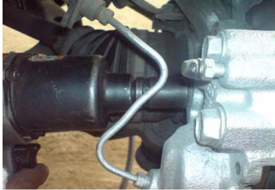
7. Ensure you use high pressure air to remove any dust and lubricate with lithium grease within the piston seal .
