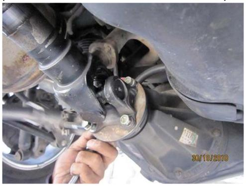
2. Clean and Bare View of the Shaft Flange View without the Bolts both Front and Rear End of the Flange.
