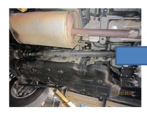
Removal Method:-First Place Notch marks on the Propeller Shaft, Yoke and the Transfer Flange. The Existing Old Shaft had already a notch which has a Yellow Paint Mark for the front and Pink for the Rear Image of the Notch Mark Sample. This was done by the Previous TSB carried out by the dealer during warranty.
