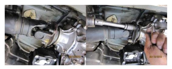
1. Remove the 4 nuts and 4 washers around the Transfer flange & Shaft yoke for the Front and Rear. Once removed this how they will look.
