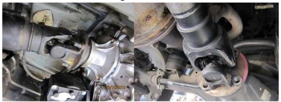
3. Now to remove the shaft, First Remove the Rear Spider Yoke End . Now just a caution, they would be a bit tight, need a Fibre / Wooden Mallet and few taps around the Flange and yoke would loose its stiffness, then you can lower it. And then go for the Front Part which is easy one. Now once shaft removed this is how they will be without the shaft. A sample View.
