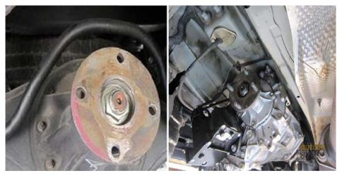
4. Now comes the Mounting Part. First Mount the Front Yoke into the Transfer Flange housing (closer to the pumpkin) and then the Rear. Mount the Bolts (total Bolts Front and Rear 4x4 = 8+ 8 washers). Align the Notch Mark which has come on the New Shaft. This is how they will look. (View of the Rear Shaft been mounted)
