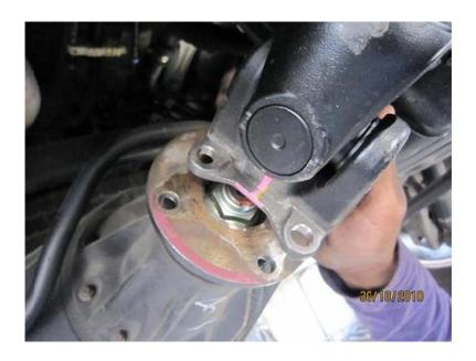
5. Now tighten the Bolts around the Flange. Torque to 88N.m(65ft.Lbf) Both Front and Rear the same specification.
