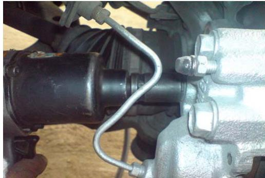
7. Ensure you use high pressure air to remove any dust and lubricate with lithium grease within the piston seal .
