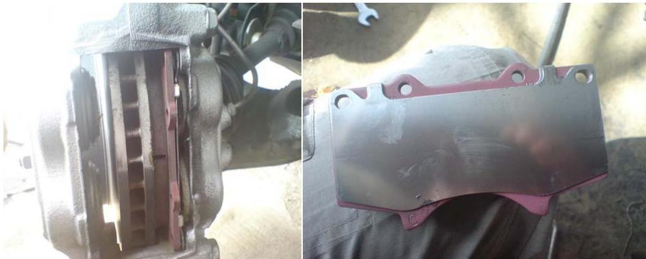
11. Install the cylinder boot and the disc brake assy. Install the front disc brake pads along with shims & the antirattle w/home pin. Same image as the "Bullet point 3"
