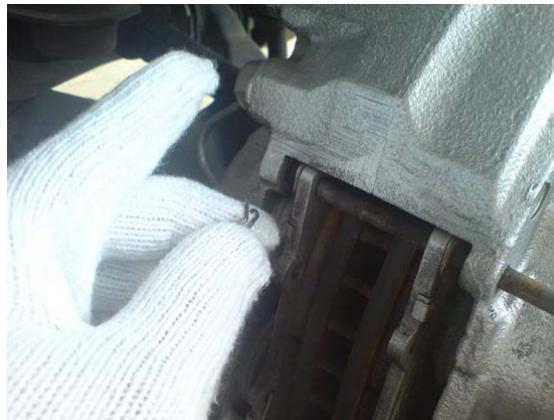
4. Remove the 2 old brake pads with anti squeal shims from the disc brake cylinder assy.
