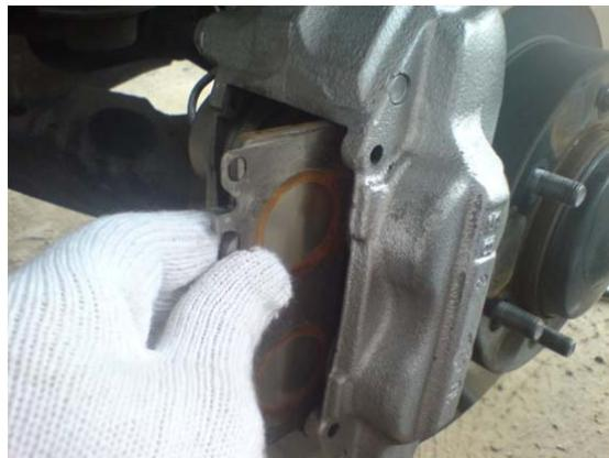
5. You do not need to remove the brake tube connected to the disc brake assy. But only remove the support clamp which is bolted to the suspension support.
