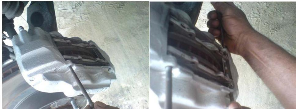
3. Remove the anti rattle spring from the disc brake pad.
