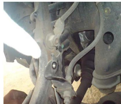
6. Remove the cylinder boot from the calliper. The last bolt is the one from the inner end which you need a torque spanner which mine was quite difficult to remove and seems was not serviced for quite sometime.
