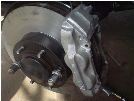
10. First retract the piston assy up into its place. A little additional pressure is required while pushing the piston in. Install the pads along with the shims. The shims comes with small pack of graphite grease. Rub a small amount on the shims so that they don't make any noise when pressure is applied while braking.
