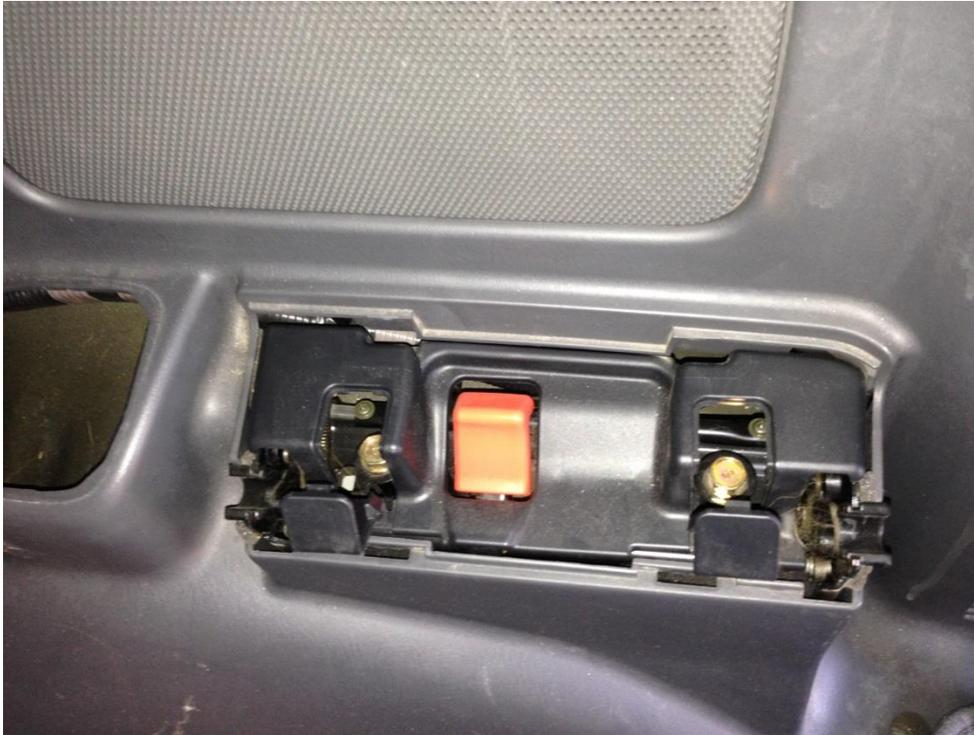
Remove the cover from the third row seat attachment, if applicable and pry back the covers on each side of the orange release button and remove the bolts. The assembly will lift out.
