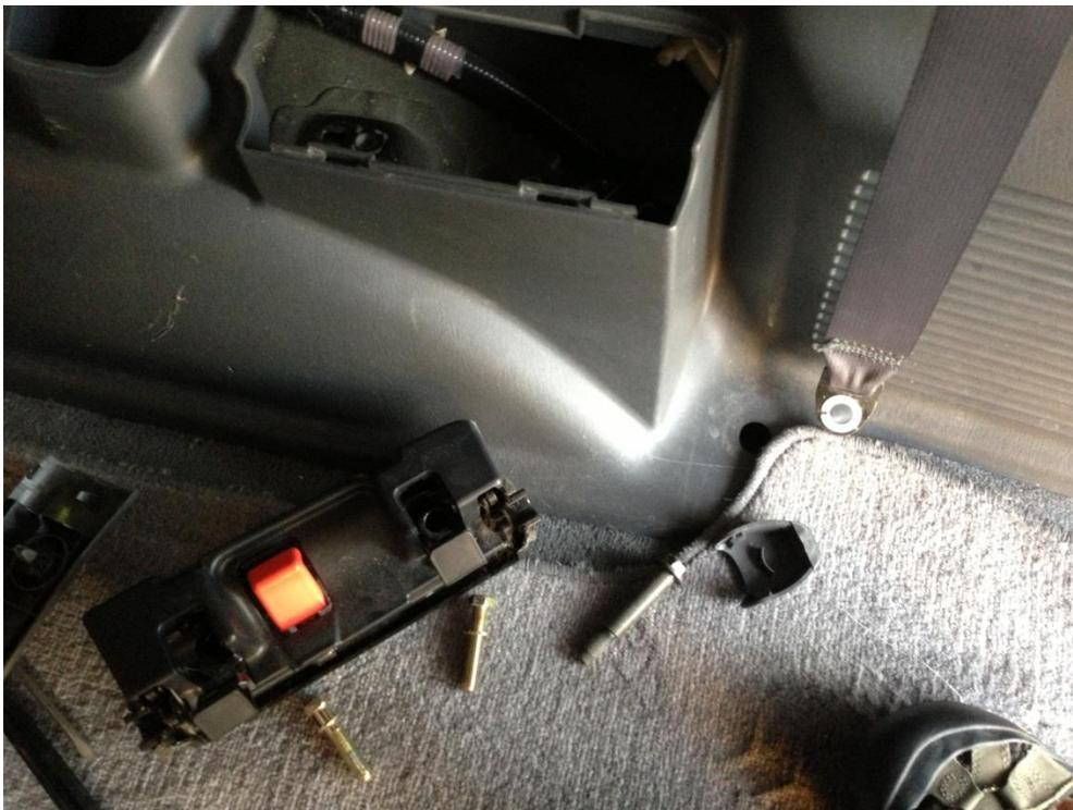
The seat belt cover prys off exposing the long bolt
