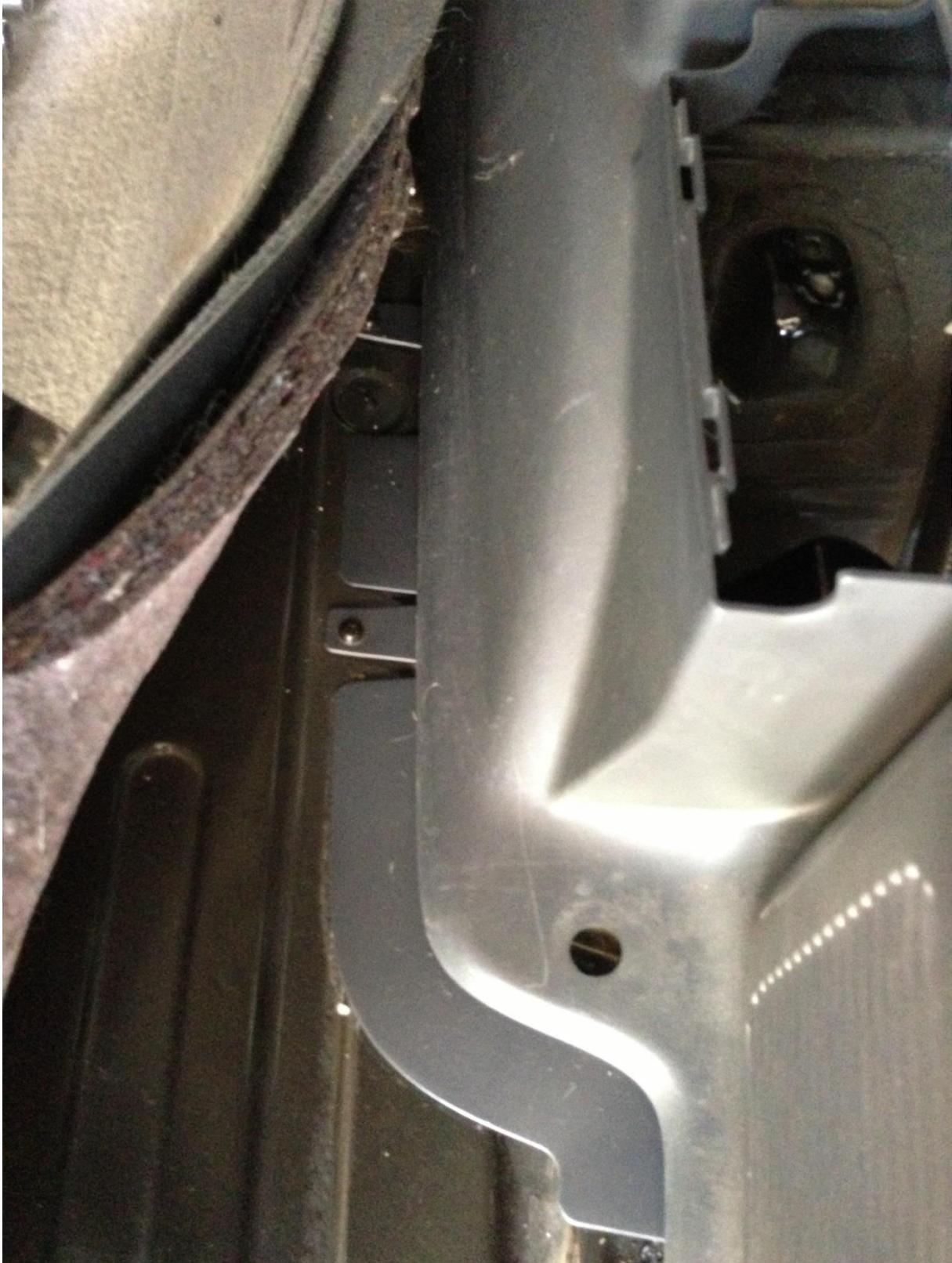
Pull back the carpet to expose the screws holding the rear side panel in place and remove the screws.
