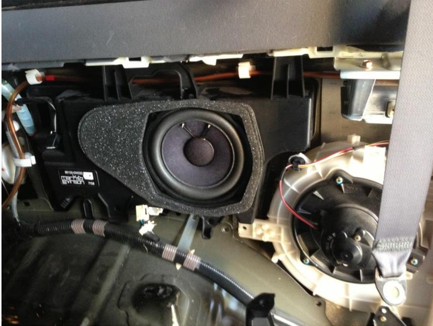
Remove the bolt and metal plate holding the rear air in place to allow the sub to be removed.
