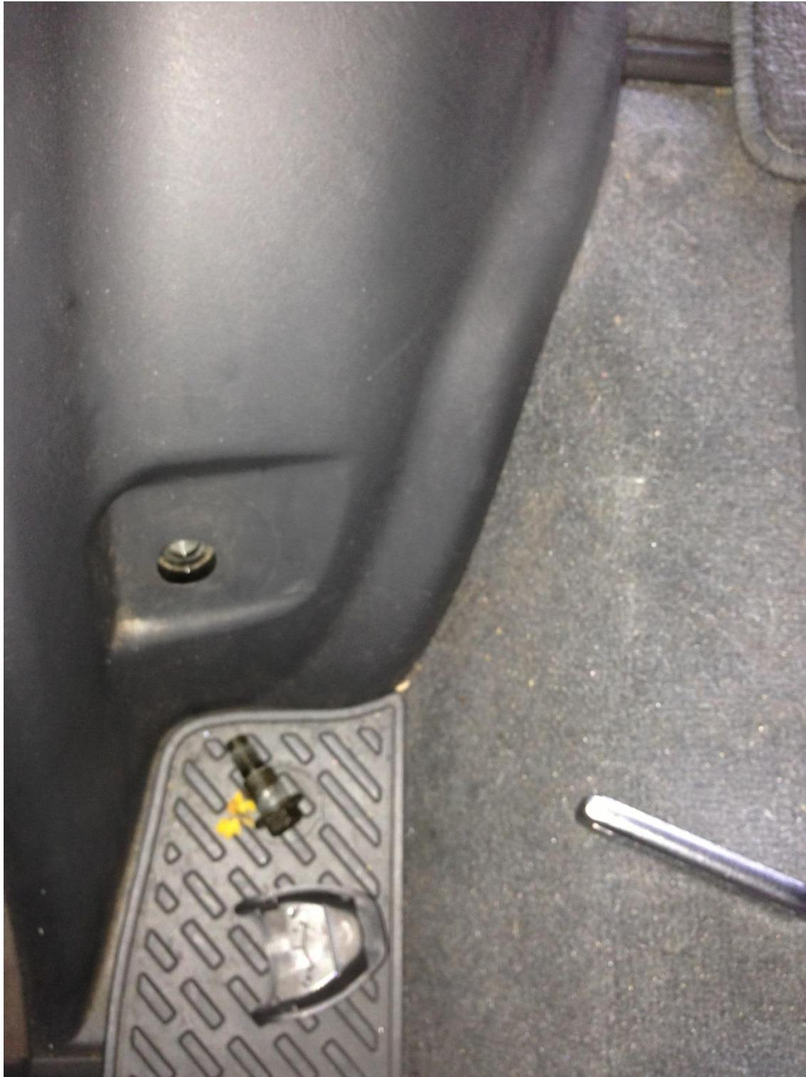
The rear passenger seatbelt, step and trim can be removed in the same fashion as the rear. The panel can now be removed, exposing the sub. There is a pug attached to the 110 outlet, so use caution not to break it when detaching.
