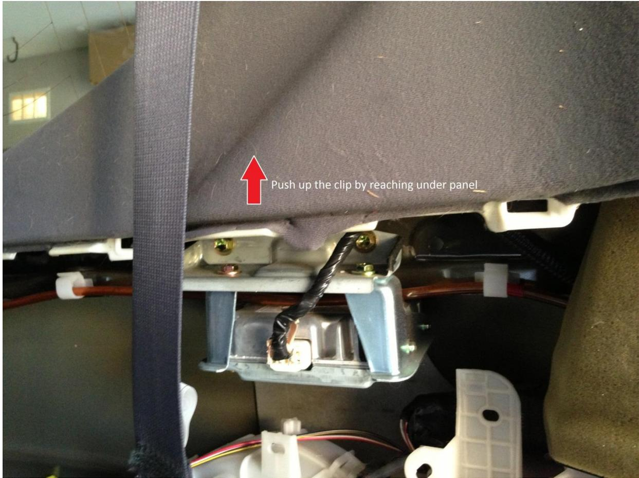
The speaker box assembly can now be removed.
