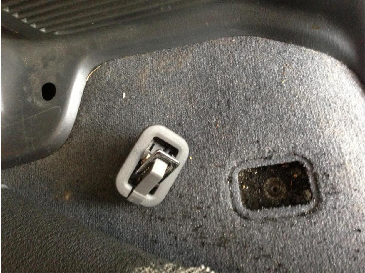
There's also a cover over the rear tie downs that simply preys up exposing the bolt. Both front and rear ones will have to be removed.
