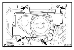
(b) Install the w/ box speaker assy No.1 with the 4 bolts. **NOTICE:**
