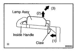
Using a screwdriver, disengage the claw and remove the (k) illumination lamp assy, as shown in the illustration.
