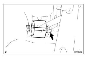
(b) Remove the nut, washer and bolt with the upper control arm assy.
