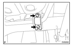
(b) Install the stabilizer bar and the 2 stabilizer brackets with the 4 bolts.
