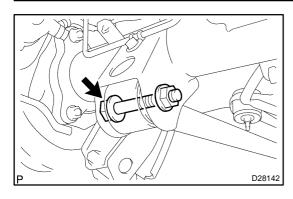
(b) Install the rear axle housing, and temporarily tighten the bolt, washer and nut.
