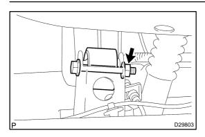
(b) Install the rear axle housing, and temporarily tighten the nut, washer and bolt.
