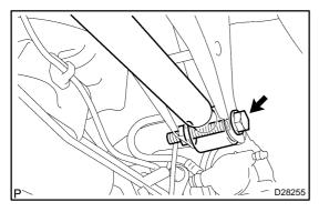
(b) Remove the bolt, nut and lateral control rod assy. HINT:
