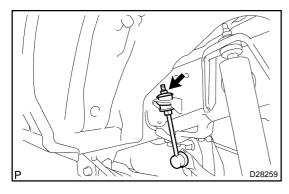
(c) Hold the stabilizer bar link with a wrench, and install the nut, retainer, cushion and link.
