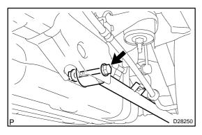
(b) Remove the nut, washer, bolt and the lower control arm assy.
