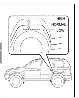
Amount of change in vehicle height: **HIGH position**40 mm (1.57 in.) **LOW position**-20 (-0.79 mm)
