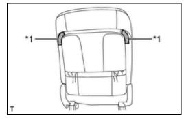
(d) Insert a screwdriver between the front seatback board subassembly LH and separate type front seatback assembly.
