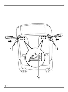
(e) Place the screwdriver at point A shown in the illustration and move the screwdriver in the direction of the arrow to detach the 2 guides and remove the 2 front seatback board clips from the front seatback board sub-assembly LH.
