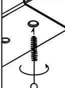
To remove debris from weldnuts in frame, spray lubricant or compressed air into hole. For heavy debris, use a small wire brush. (Be careful not to damage threads).
