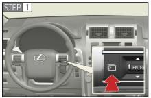
Press and hold the button on the steering wheel to display vehicle customization mode.
