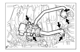
**d.** Using several steps, uniformly tighten the 2 bolts and 4 nuts in the sequence shown in the illustration.
