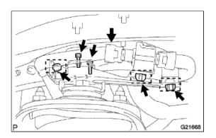
**c.** Using SST, remove the nut and bracket.
