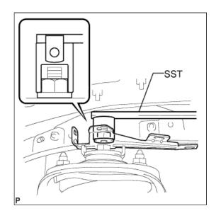
**d.** Remove the bolt, nut and washer.
