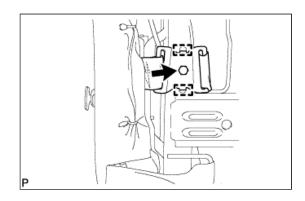
**b.** Remove the hog rings and detach the hooks, and then remove the seatback cover with pad.
