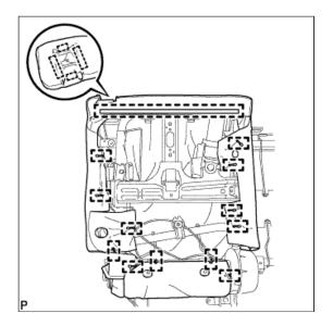
**c.** Disconnect the outer belt from the seatback cover with pad.
