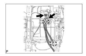
**c.** Detach the hook and remove the seat cushion cover with pad.
