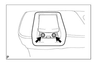
**b.** Disconnect the cable in the order shown in the illustration and remove the lever.
