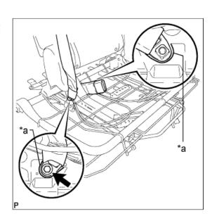
**a.** Install the center seatback with the 2 bolts.
