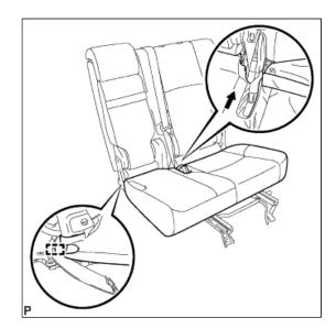
**c.** Attach the hooks to install the seat cushion cover with pad.
