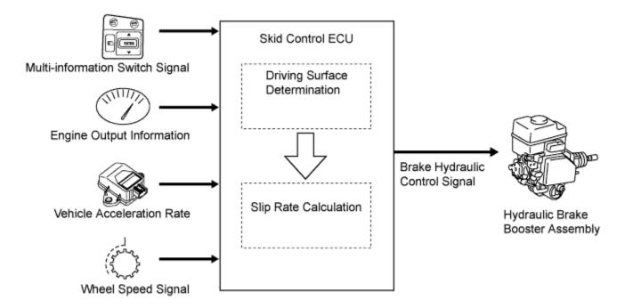
Brake Hydraulic Pressure Control Image of Multi-terrain ABS
