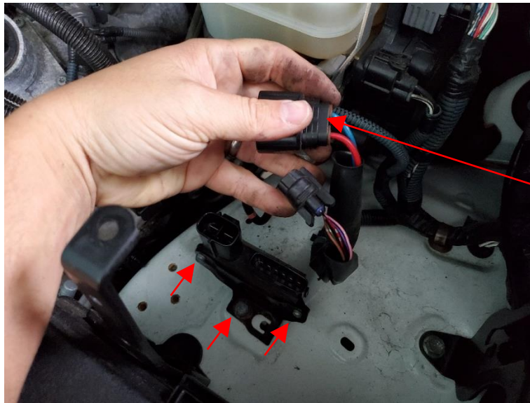
Figure 3 - Remove the Factory AID and Replace with the Gen-II Module
