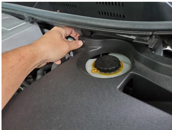
Figure 2 - Removing the Driver's Side Engine Bay Cover
