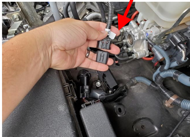
Figure 7 - Connect the Gen-II ASV Harness to the Gen-II Unit
