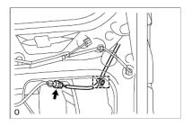
$\mbox{\bf d.}$  Using a screwdriver, detach the 5 claws and remove the outside garnish.
