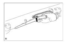
**b.** Detach the 2 claws and remove the washer nozzle.
