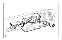
**b.** Remove the 4 bolts and back window glass.
