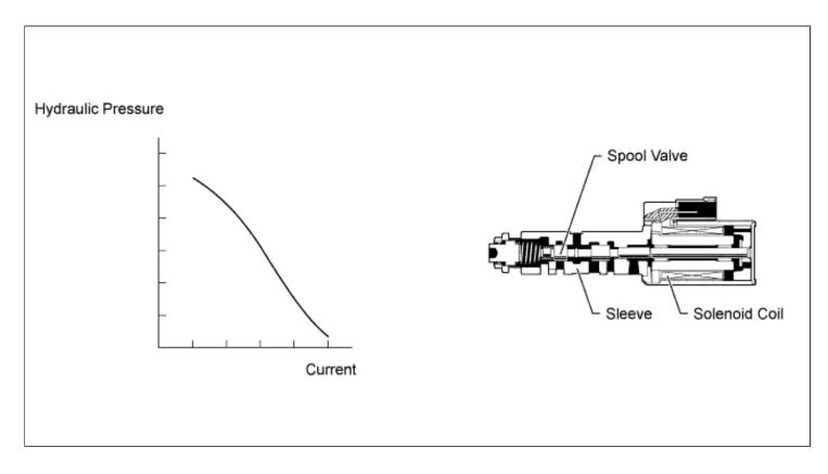
Shift solenoid valve SLT controls the transmission line pressure for smooth transmission operation based on signals from the throttle position sensor and vehicle speed sensor. The ECM adjusts the current to shift solenoid valve SLT to control the hydraulic line pressure coming from the primary regulator valve. Appropriate line pressure assures smooth shifting with varying engine outputs.
