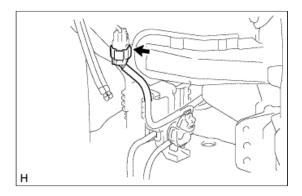
**b.** w/ Headlight Cleaner System: Disconnect the 3 connectors.
