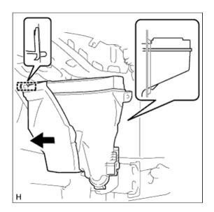
8. REMOVE WINDSHIELD WASHER MOTOR AND PUMP ASSEMBLY
