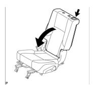
(g) Operate the rear seat track adjusting handle to move the seat to the center position.
