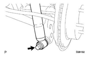
**c.** Remove the bolt and disconnect the rear shock absorber assembly LH from the rear axle housing.
