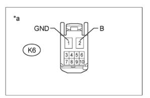
c. Measure the resistance according to the value(s) in the table below.
