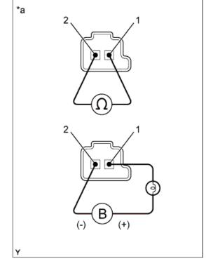
**c.** Apply 12 V battery voltage to the shift solenoid valve and check that the valve moves and makes an operating noise.
