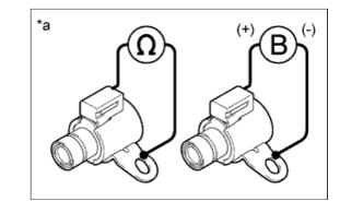
c. Apply 12 V battery voltage to the shift solenoid valve and check that the valve moves and makes an operating noise.
