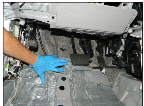
Figure 6. Driver Side Dash Panel Insulator Assembly Inspection
