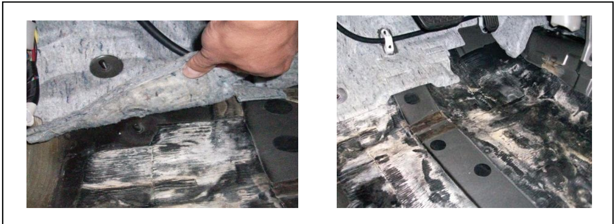
Figure 5. Examples of Organic Matter Growth Due to Water Intrusion Found During Vehicle Inspection
