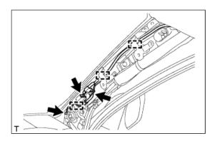
**g.** Disconnect the 2 connectors and detach the clamp from the rear pillar LH.
