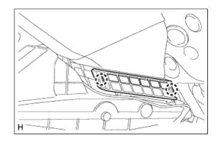
**b.** Swing the bottom of the duct sideways and remove the duct.
