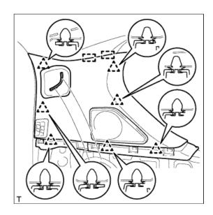
**c.** Detach the 4 clips and 2 guides, pass the rear No. 2 seat outer belt floor anchor through the rear quarter trim panel and remove the rear quarter trim panel.
