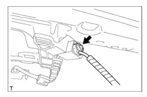
**k.** Remove the roof headlining from the back door as shown in the illustration.
