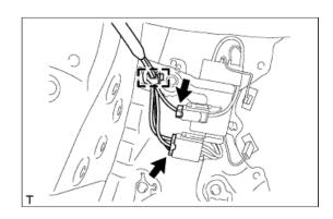
**h.** Disconnect the connector and detach the 3 clamps from the rear pillar RH.
