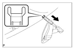
**b.** Detach the 2 claws and remove the inner rear view mirror stay holder cover.
