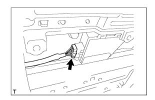
**d.** Disconnect the 2 connectors and detach the 3 clamps from the front pillar LH.
