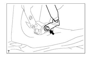
e. Disconnect each connector and remove the deck trim side panel.
