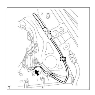
i. Detach the 2 clips, 2 guides and 8 fasteners.
