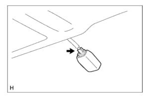
**c.** Disconnect the drive gear connector.
