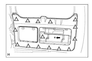
a. Remove the 4 bolts and 2 tool box brackets.
