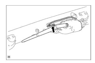
**b.** Detach the 2 claws and remove the washer nozzle.
