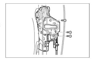
**c.** Disconnect the cable and remover the back door lock assembly.
