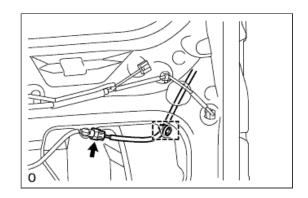
**d.** Using a screwdriver, detach the 5 claws and remove the outside garnish.
