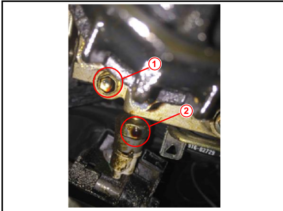
Figure 1. Oil Leak From Engine Oil Pressure Sensor
