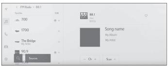
[Ch]: Touch [ - ] or [ + ] to search for the receivable broadcasting stations. Touch and hold to jump to the next frequency with available radio signal. When released, the broadcasting station closest to that position with the best reception sensitivity is selected automatically.
