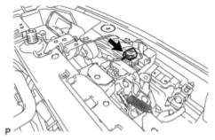
(j) Disconnect the connector. (w/o Wide View Front Monitor System)
