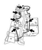
(a) Remove the 6 bolts and No. 1 radio bracket.
