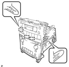
(a) Disengage the 2 claws and 2 guides to remove the radio receiver assembly from the integration control and panel assembly.
