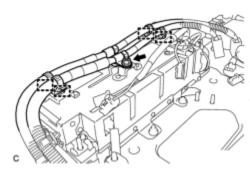
(a) Remove the nut, disengage the 4 clamps and disconnect the wire harness from the hybrid vehicle converter.
