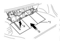
(g) Cut and shape a piece of cardboard so that it fits the area between the HV battery bolt attachment positions, and then insert it as shown in the illustration.
