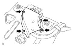
(a) Remove the 4 nuts and hybrid battery service plug cover.
