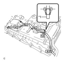
(a) Disengage the 2 claws and remove the HV battery thermistor.
