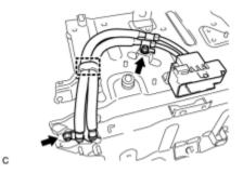
(d) Remove the 2 nuts, disengage the clamp and separate the wire harness from the HV battery.
