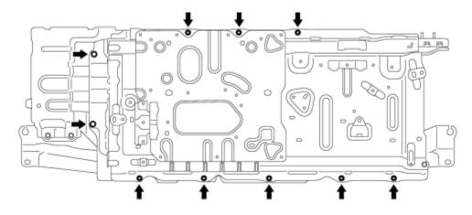
(b) Remove the 2 bolts and 2 bushings with the 2 washers.
