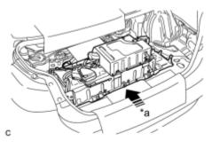
(c) Push the HV battery together with the cardboard toward the front of the vehicle.
