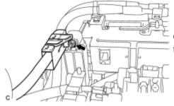
(a) Remove the nut and disconnect the frame wire from the inverter terminal.
