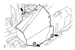
(a) Remove the 2 bolts, nut and front hybrid battery shield.
