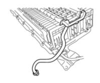
(a) Remove the hybrid battery hose assembly from the HV battery.
