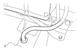
(d) Remove the grommet and hybrid battery hose assembly.
