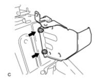
(b) Remove the 2 nuts and upper hybrid battery cover sub-assembly.
