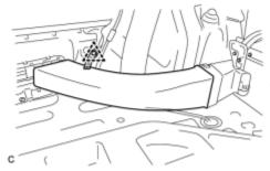
(a) Remove the clip and No. 2 hybrid battery exhaust duct.
