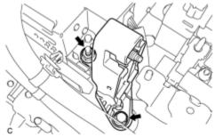
(b) Remove the bolt, nut and inverter terminal.
