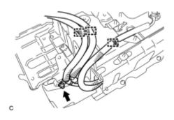
(a) Remove the nut, disengage the 3 clamps and disconnect the wire harness from the HV battery.
