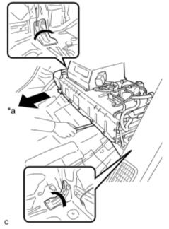
(i) Use a tire lever from the cabin side to lift the HV battery up over the tabs on the body.
