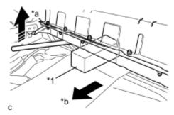
(j) Using a tire lever to hold up the HV battery, insert a wooden block or equivalent as shown in the illustration.
