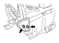
(a) Remove the 2 nuts and rear No. 1 hybrid battery shield.
