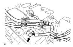
(d) Disconnect the connector and 4 clamps and remove the No. 2 hybrid battery pack wire.
