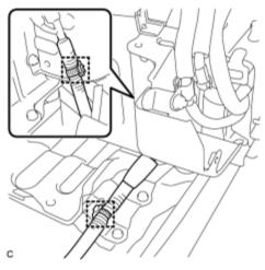
(a) Disconnect the 2 clamps from the HV battery shown in the illustration.
