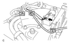
(c) Disconnect the connector and 3 clamps from the HV battery shown in the illustration.
