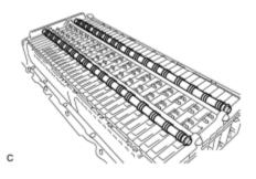
(a) Remove the No. 1 battery insulator duct from the HV battery.
