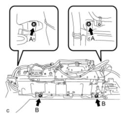
(f) Install the 4 bolts to the HV battery.
