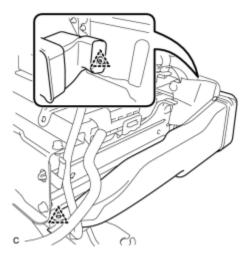
(a) Remove the 2 clips and No. 1 hybrid battery exhaust duct.
