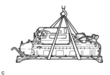
(m) Using a suitable adaptor such as a rope, remove the HV battery while tilting the HV battery.
