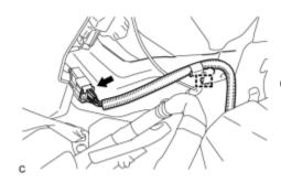
(c) Disconnect the battery pack wire connector and clamp.
