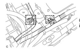
(b) Disconnect the 2 clamps from the HV battery shown in the illustration.
