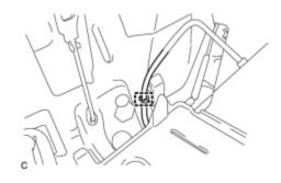
(b) Disconnect the battery room ventilation hose.
