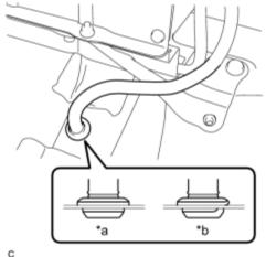
(g) Connect the battery room ventilation hose with the grommet.
