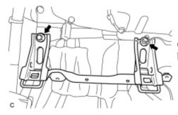
(b) Remove the 2 bolts and child restraint seat anchor bracket sub-assembly RH.
