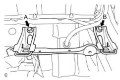
(a) Install the child restraint seat anchor bracket sub-assembly LH with the 2 bolts.
