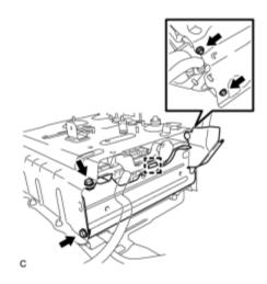
(a) Remove the 3 bolts, nut, guide and No. 2 hybrid battery shield sub-assembly.
