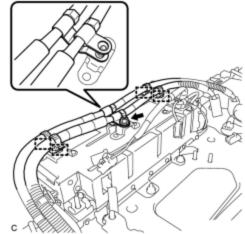
(c) Connect the wire harness with the nut and 4 clamps to the hybrid vehicle converter.
