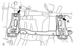
(a) Install the child restraint seat anchor bracket sub-assembly RH with the 2 bolts.
